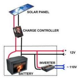
connected in series. They have a capacity of 12v/100amp/hrs each. A power drain of 240 watts per hour is estimated. That means the batteries could provide up to 10 hours of runtime (2400
