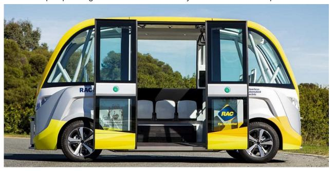
The <u>Navya</u>, one of several options, has15 seats and no steering wheel. The automated electric tram requires no overhead power. Rubber tires enable it to travel on ordinary streets.
